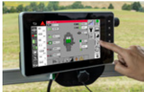
Standard Electronic Bale Length Control operates via the Fieldstar 5 baler terminal.
