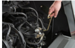
The knotter head can easily be lifted for inspection and service.
