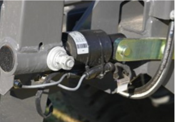
◀ Accurate load cells for the integrated bale weighing system.
