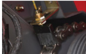
Automatic lubrication for the drive chains is fitted as standard.
