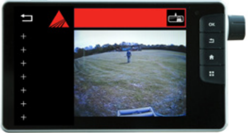
▲ Rear Video Camera provides the best possible information and awareness of what is happening at the back of the baler.
