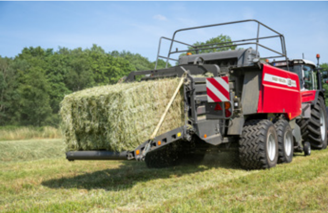
▲ Electronic Bale Weight Kit - in addition to live data, the average weight and field total weight is saved in the job records location.
