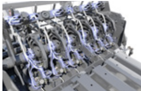
AutoLube increases knotter reliability and reduces maintenance.
