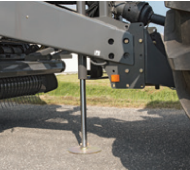
▲ Hydraulic park jack - for faster and safe hitching up.
