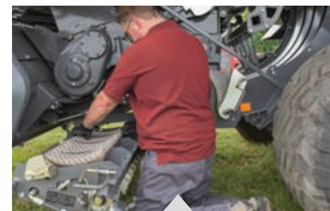
Ample accessibility offering straightforward knife removal
