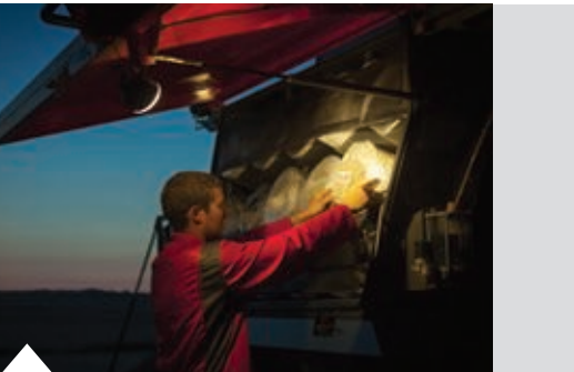
Twine box lighting allows easy night time refilling.
