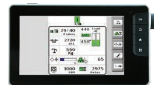
Automatic density control through the FieldStar 5 baler terminal.
