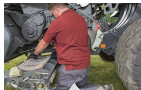
Ample accessibility offering straightforward knife removal
