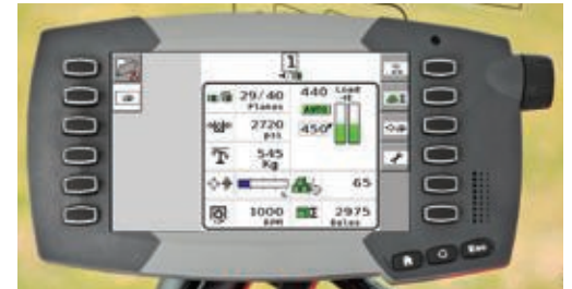
Automatic density control through the C1000 Baler Monitor.
