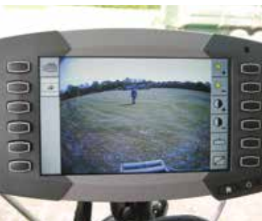
A video camera can be easily added to your pre-wired baler. The C1000 Baler Monitor is full colour video compatible as standard.
