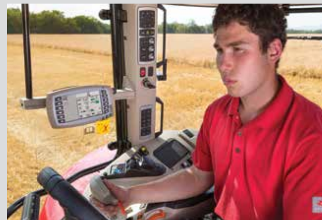
Controlling the baler via the tractor ISO VT terminal.
