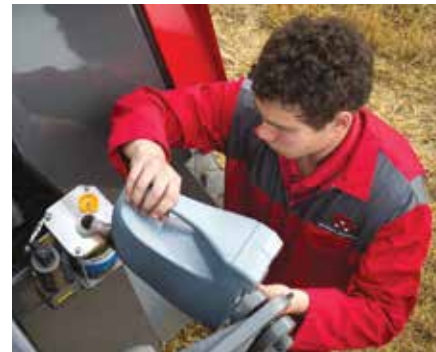
Refilling the automatic chain oiler.
