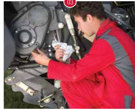
Checking the cutter gearbox oil level.
