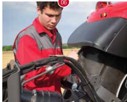
Greasing the PTO shaft.
