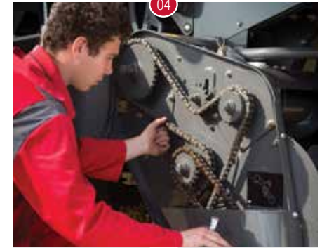
Checking the pick-up chain tensions.
