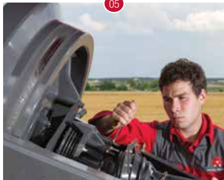
Adjusting the flywheel slip clutch.
