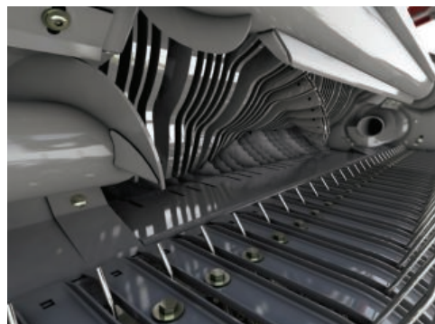
A full width auger is fitted on the 'Cutter' balers.
