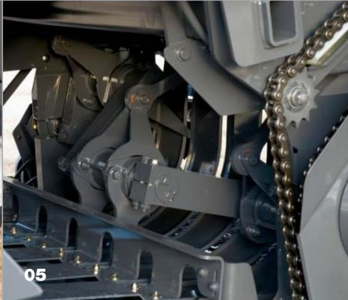
**05** Packer crank = Even feed into pre-pack chamber.
