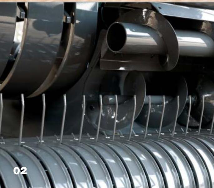
**02** Four feeding augers = Higher capacity feed.
