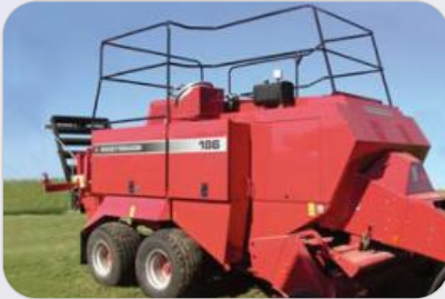
The MF 186 produces bales of 0.70 m x 1.20 m section up to 2.50 m long and will bale silage, hay and straw.
