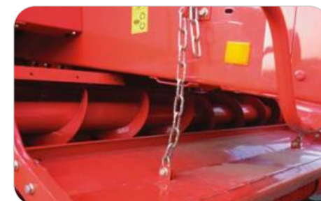
MF185 SII, MF186 and MF187 balers have a solid high performance windguard for smooth crop flow.
