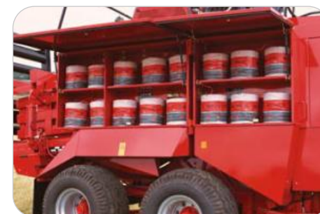
There is plenty of room for twine storage on each side of the baler.
