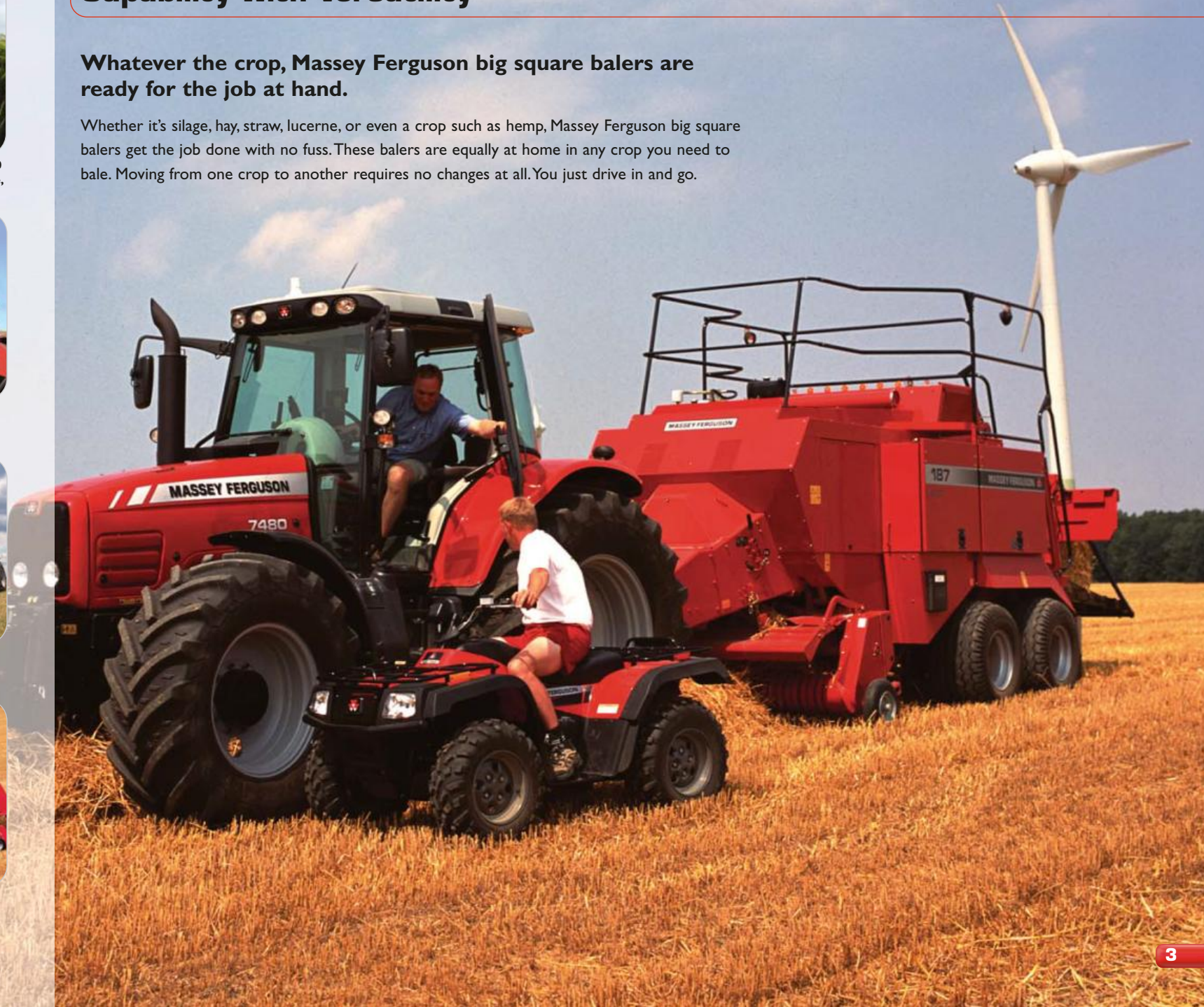
The MF 186 produces bales of 0.70 m x 1.20 m section up to 2.50 m long and will bale silage, hay and straw.
