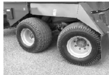
Optional self-steering tandem axle turns up to 19 degrees. Can be locked out for reversing and road travel
