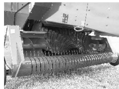
Optional cutter unit with 4 lobed rotor and 19 knives give as low as 48mm chop length
