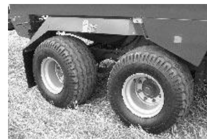
Optional self-steering tandem axle turns up to 19 degrees. Can be locked out for reversing and road travel
