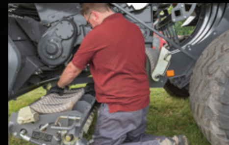
▲ Ample accessibility offering straightforward knife removal
